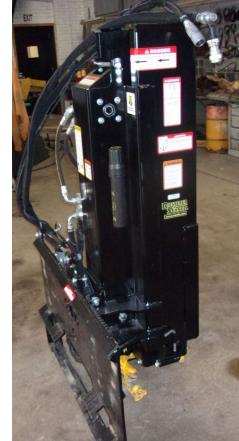
A close-up view of the black mechanical components of the post pusher/puller, showing hydraulic hoses and structural details. |
