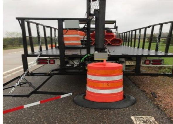
A black metal trailer with a hydraulic lift system. A red and orange striped traffic barrel is being lifted onto the trailer. A red and white striped barrier is on the ground in front of the trailer. |
