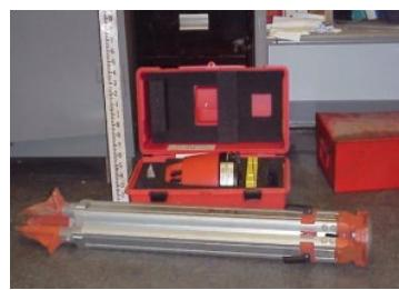
A red and silver laser transit instrument in its carrying case, with a tripod and a survey rod visible in the foreground.                                                |                                                                                                                                                                                                                                                          |
