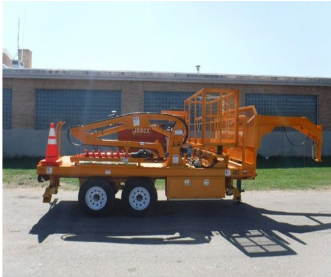
Class 9428 Sign Trailer, with auger and lift
