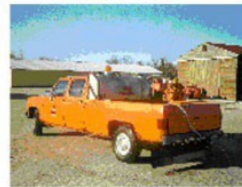
Class 9255 Spray Bar Applicator, multiple purpose, including anti-icing liquid application system, without ground speed controller, to include tank, spray bar, pump, nozzles and hardware (either slide in, stand alone or pull behind) with tank size from 0 to 499 gallons
