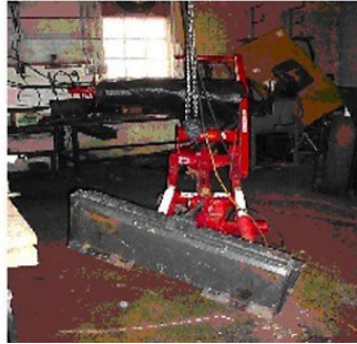
Class 9240 Fence Installer (for silt)
