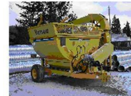
Class 9012 Bale Chopper or Mulcher, 25 hp or greater or PTO
