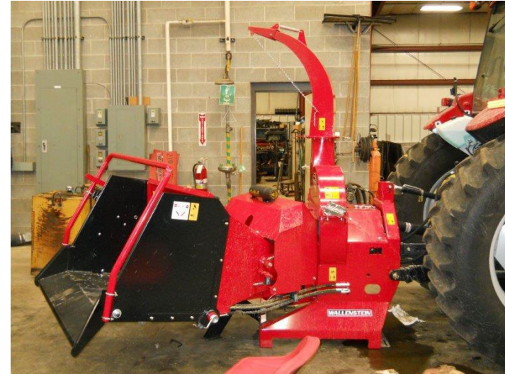
Class 9406 Brush Chipper, 3 point tractor mounted
