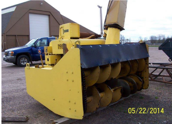
Class 9404 Snow Blower, rotary, powered by engine, uses motor fuel
