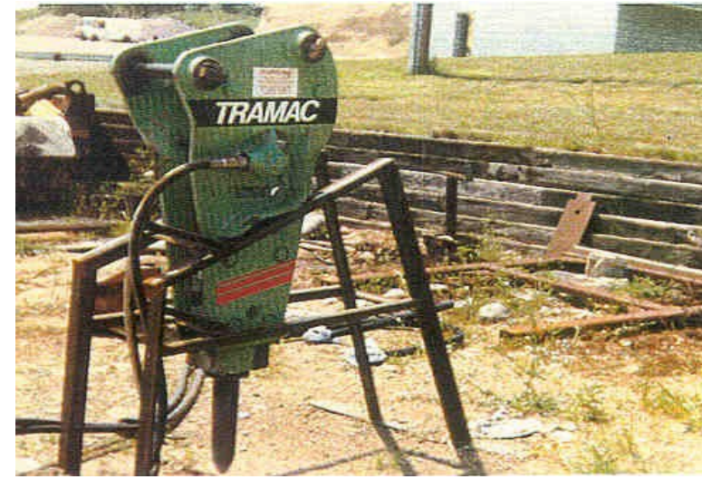
Class 9054 Hammer, hydraulic, 100 thru 1100 ft/lbs, CIMA rating
