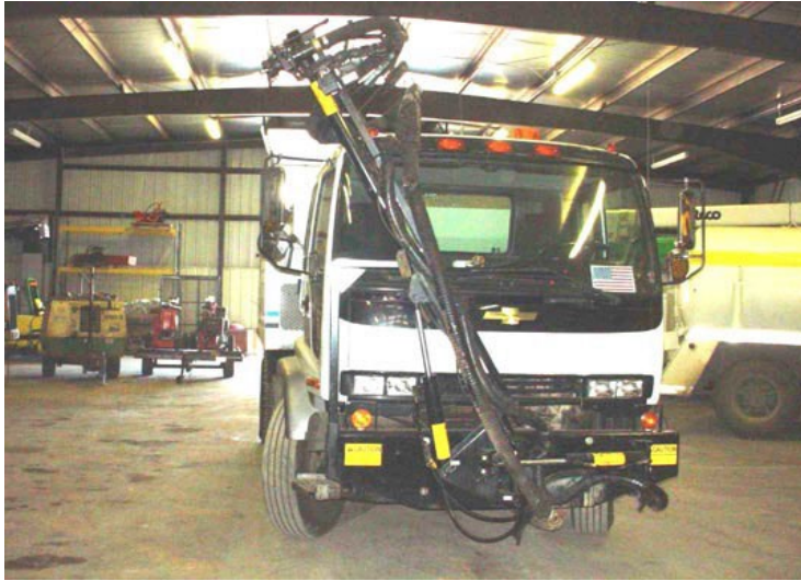
Class 9082 Pothole Patcher, spray injection, truck mounted, single unit
