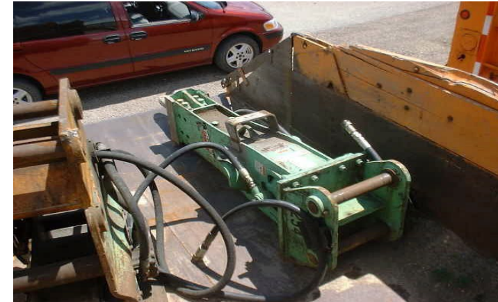
Class 9254 Hammer, hydraulic, 1101 ft/lbs and over CIMA rating
