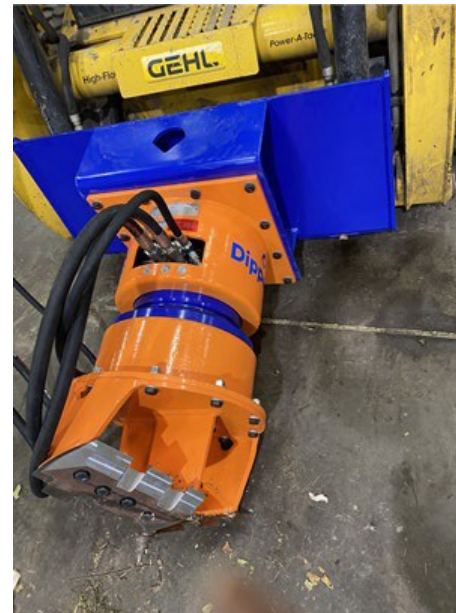
Class 9152 Stump Grinder, Hydraulic
