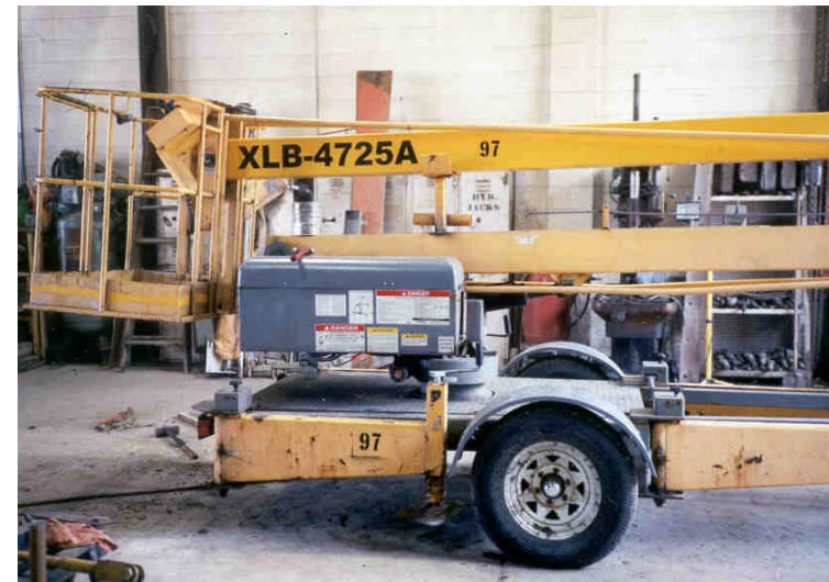
Class 9312 Boom Lift, towed on own trailer
