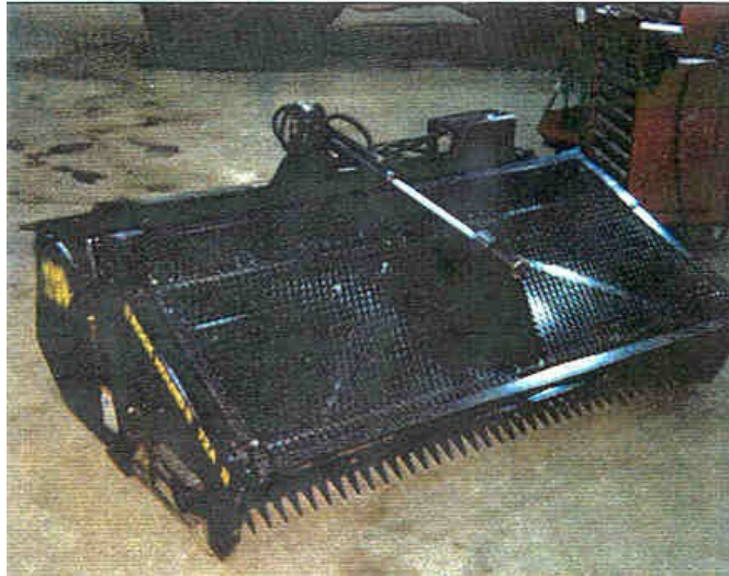
Class 9113 Rake, rock/Hydraulic Grapple
