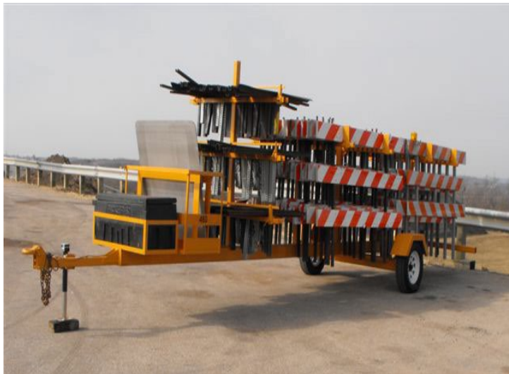
Class 9389 Emergency response trailer – open trailer for transporting supplies and tools to the incident
