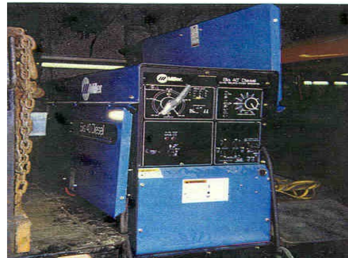
Class 9286 Welder and Generator (engine driven)
