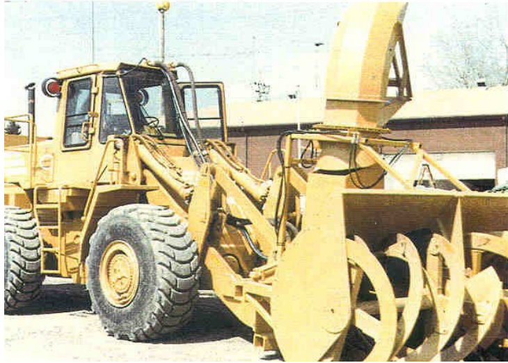
Class 9095 Snow Blower, rotary, hydraulic or PTO driven, does not use fuel
