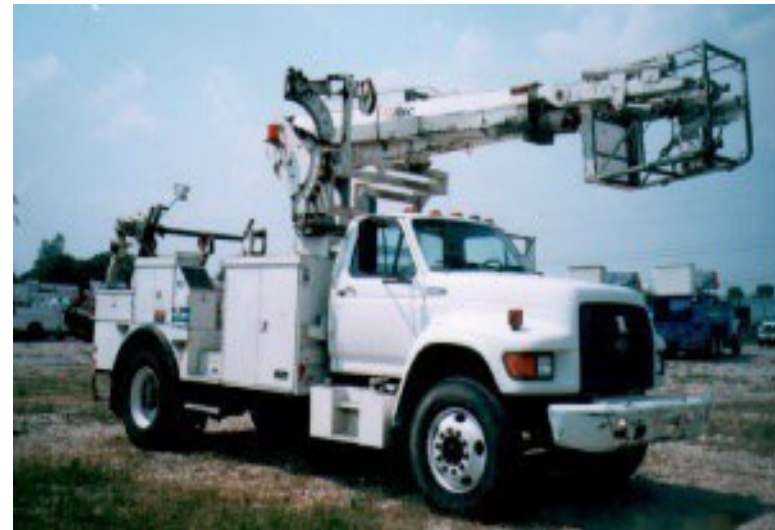
Class 9070 Crane, Hydraulic (Truck Mtd.)
