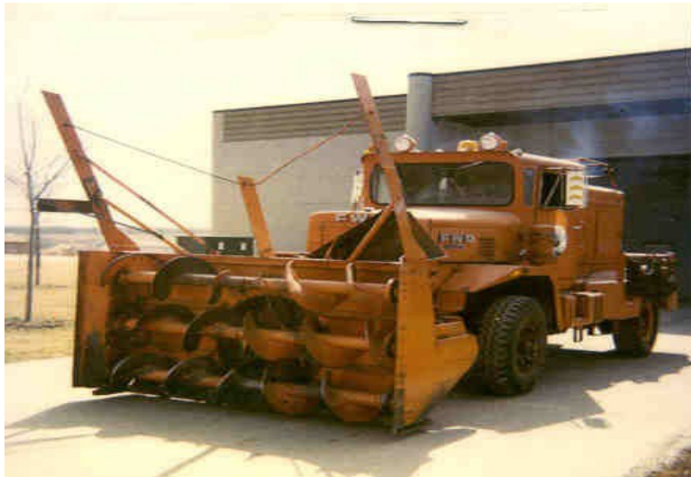
Class 9296 Snow Blower, powered by engine, rotary plow, integral unit, used exclusively for snow plowing and uses motor fuel
