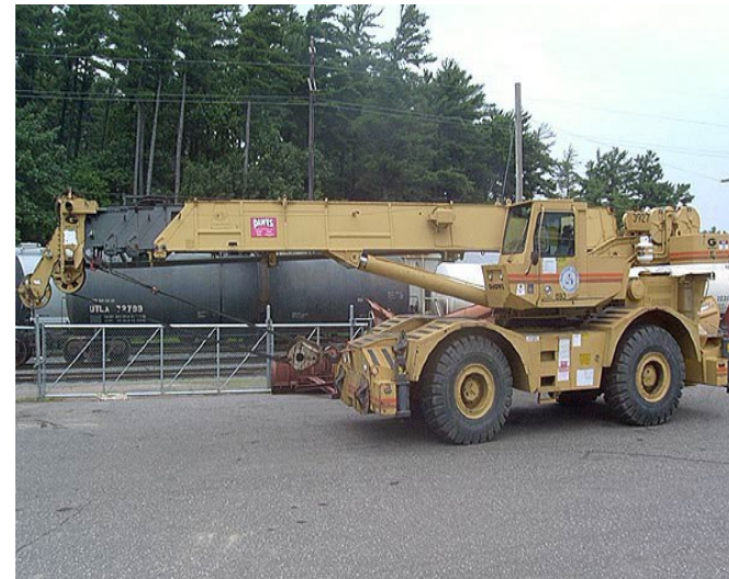
Class 9020 Crane, 45 tons, 104' boom
