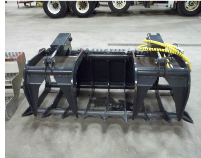
Class 9113 Rake, rock/Hydraulic Grapple
