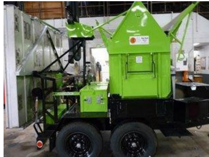
Class 9410 Infrared Asphalt Heater, trailer mounted
