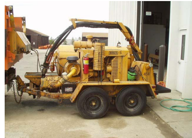
Class 9081 Patch Machine, spray-injection, trailer mounted
