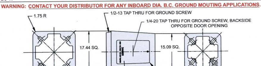
BOTTOM BOLT CIRCLE FOR 17 1/4" DIA. B.C. 4 PLS. EQ. SPACED USE 2 3/4" DIA. X 1 5/16" I.D. X 1/2" TK. STEEL WASHERS
