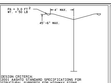
DESIGN CRITERIA: 2001 AASHTO STANDARD SPECIFICATIONS FOR STRUCTURAL SUPPORTS FOR HIGHWAY SIGNS, LUMINAIRES. AND TRAFFIC SIGNALS.
