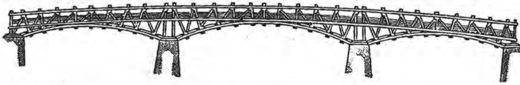
A. Timothy Palmer's "Permanent Bridge" over the Schuylkill River, Philadelphia. Built in 1804, the bridge had a middle span of 195 feet, and side spans of 150 feet each.
