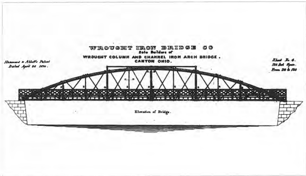
Figure 15: General plan for overhead bowstring truss bridge, by Wrought Iron Bridge Company, 1870. The company built a bridge of similar design in Oconomowoc, Waukesha County, in 1872. (Source: WisDOT).
