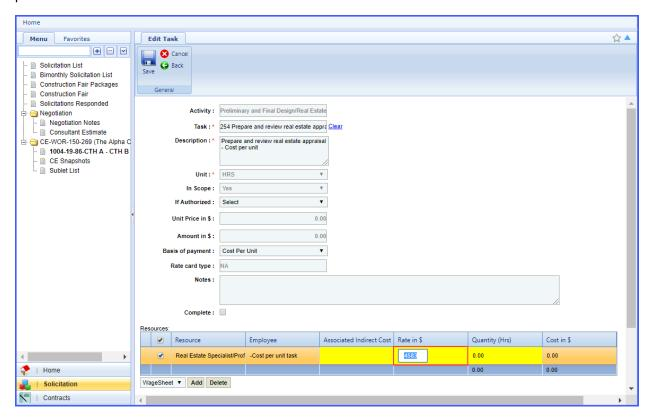
Double-click in the **yellow cell** under the Quantity column and enter 1. Click **out of the cell** so that a red triangle appears in the upper-left corner of the cells under the Rate in \$ and Quantity columns. The Cost in \$ will now calculate.
