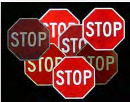
to maintain retroreflectivity. Properly maintained retroreflectivity improves nighttime conspicuity and visibility. Signs installed to conform to the MUTCD are expected to result in a crash reduction of 15 percent for injury collisions and 7 percent for PDO collisions
