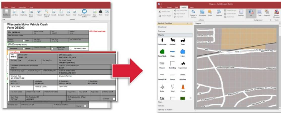
This feature can be set as a default by a TraCS Administrator using TraCS Office. In the Distribution (Configuration Wizard) Form, there will now be an option to set client computers to automatically set the TLT image chosen in the **Location** section of the crash form as the Diagram Tool background.
