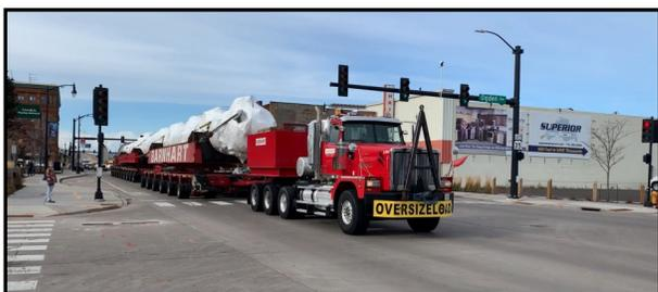
On the evening of Dec. 1, the Barnhart crew began the trek from Fraser to a laydown yard on Stinson Avenue at 7 p.m. using the Goldhofer, which is controlled by an operator walking in front or behind it, Smith said. Moving at walking speed and adhering to the cable restrictions, the column made it to its final destination just before 2 a.m. Dec. 2.
