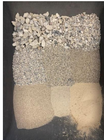
Figure 3.13 Gradation controlled sample preparation
