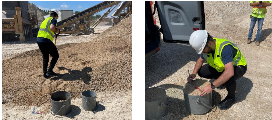
Figure 3.8 Unit box test: (a) filling, (b) leveling
