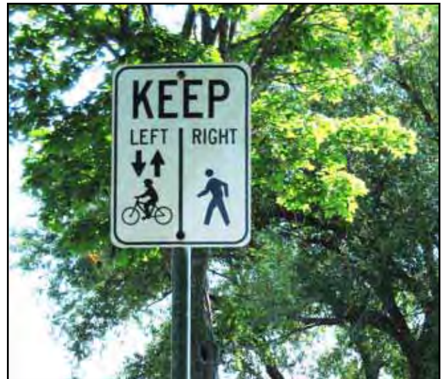
Exhibit 5-89: Designated use lane on multi-use paths keep pedestrian traffic separated from cyclists who travel at faster speeds.
