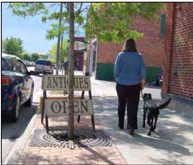
Exhibit 5-23: Combining a concrete walking area with brick edging can create a stable and attractive sidewalk corridor.
