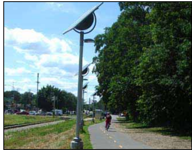
Exhibit 5-86: Solar lighting can be used on shared-use paths to provide acceptable luminance levels.
