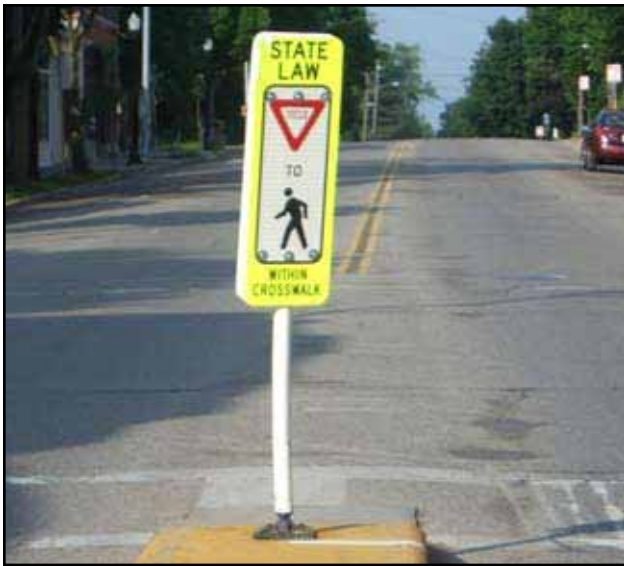
Exhibit 5-60: In-street pedestrian signs are used to alert motorists of pedestrian crossings.
