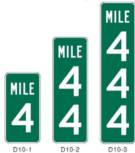
Figure 2H-2. Reference Location Signs
