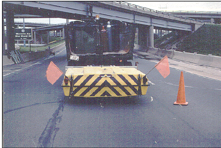
Figure 1.4.8.3-1: Truck Mounted Crash Attenuator.
