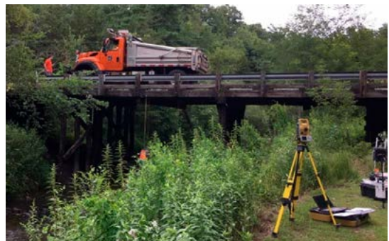
Truck parked at position of maximum strain response for survey data collection
