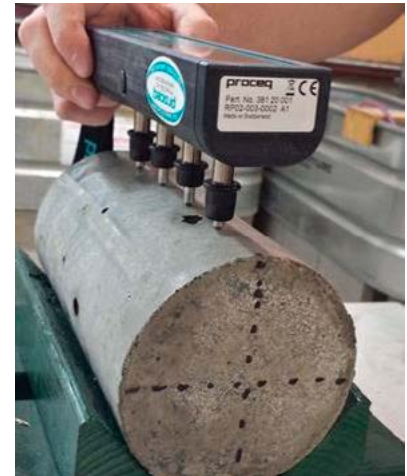
Conducting a surface resistivity test
