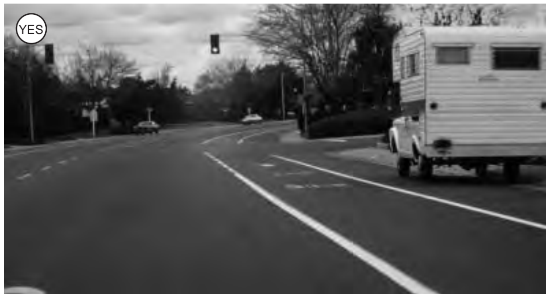
Fig. 3-4: The proper location for a bicycle lane is to the left of the parking lane. In this location, bicyclists and motorists can clearly see each other.
