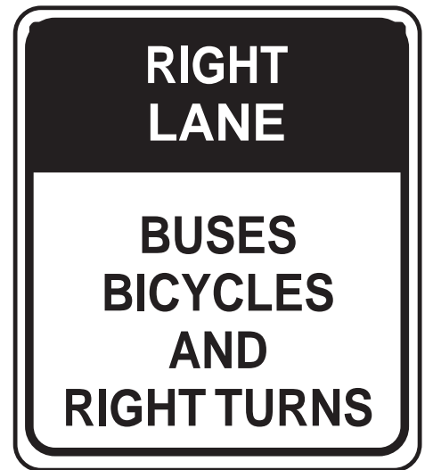
Figure 3-18: Signing and marking for a combination lane should clearly identify its purpose.
