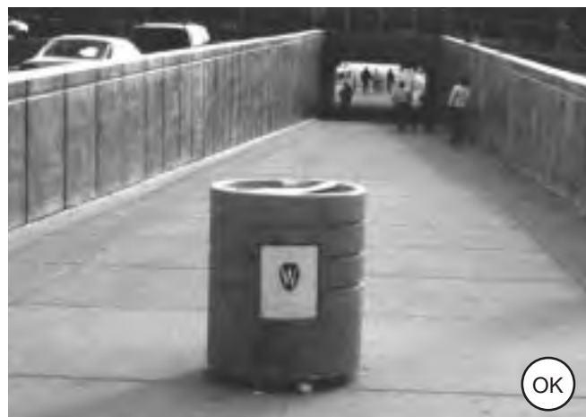
Figure 4-154: In well-lit areas, street furniture like decorative garbage cans can work better than bollards.
