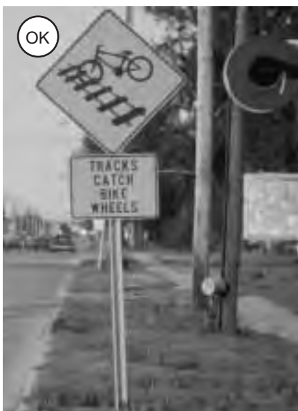
Fig. 2-44: Warning sign W11-59.3 (similar to that shown) may be used where the hazard cannot be completely eliminated.
