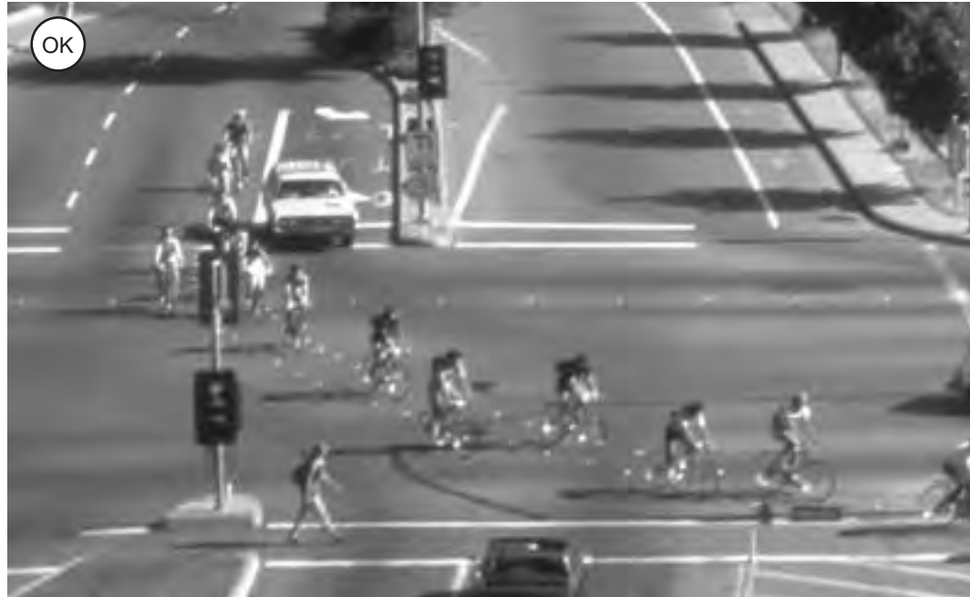
Figure 3-43: As shown in this illustration, dashed lines may be used to lead bicyclists to the destination bicycle lane.
