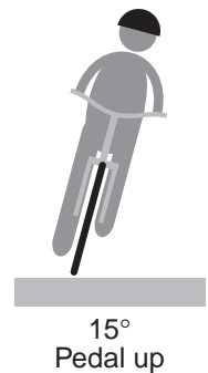
Figure 4-22: Bicycles turn by leaning. Too much lean can cause a “pedal strike.” Tricycles turn by steering.
