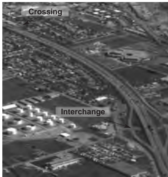
Figure 2-61: The non-interchange crossing provides a lower-volume and easier freeway crossing for bicyclists than the interchange.
