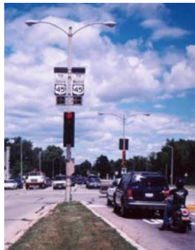
Figure 25.3-1: Trailblazer Placement at Intersection
