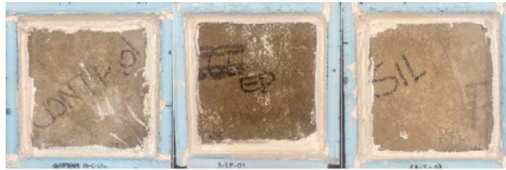
Deicer scaling specimens before testing (from left to right: A-FA Control, A Epoxy, A-FA Silane)
