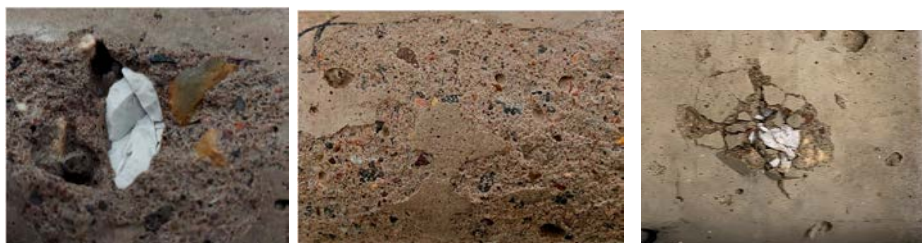
Photos of PCC cylinders during F-T cycles showing the effect that CA quality had on the cylinders. Photos show CA fracture, PCC surface scaling and CA initiated cracking in the PCC cylinder surface, respectively.
