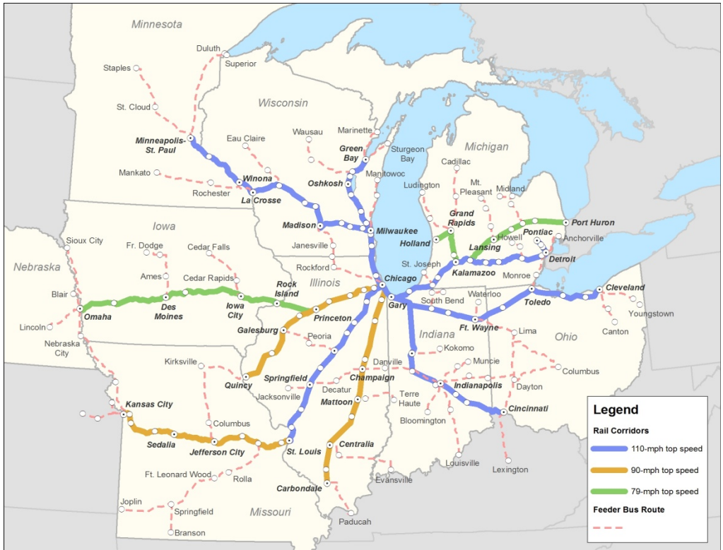
Map 6-4: Proposed Midwest Regional Rail System (from 2004 Midwest Regional Rail Initiative Business Plan Executive Report). Note: Actual route alignments and stations will be determined during environmental and engineering studies which will include coordination with local units of government and public involvement opportunities.
