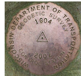
Figure 2. Geodetic survey control station
