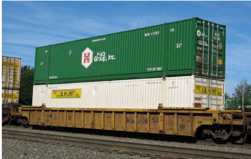
Image 7: Hub Group and J.B. Hunt 53' Intermodal Containers in Well Car (Source: RRPictureArchives.Net; photo by Gary Walton).
