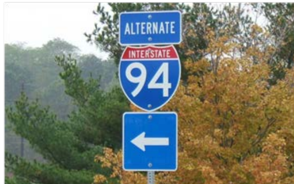
Figure 13.1 - Emergency Alternate Route Signing
